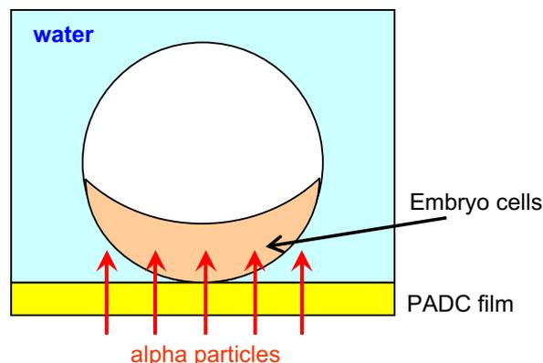
Fig. 1. Schematic diagram showing alpha-particle irradiation of a zebrafish embryo, with the embryo cells resting on the bottom, and assuming that the alpha particles strike the PADC film vertically.
