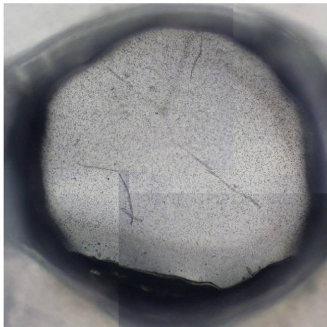
Fig. 3. An overall image of a PADc film at the bottom of the hole with visible alpha-particle tracks, reconstructed from four images covering different areas.
