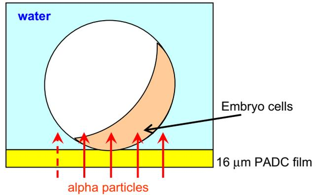
Fig. 6. Schematic diagram showing alpha-particle irradiation of a tilted zebrafish embryo. The alpha particle represented by the dashed arrow does not hit embryo cells and should therefore be discarded when calculating the radiation dose.
