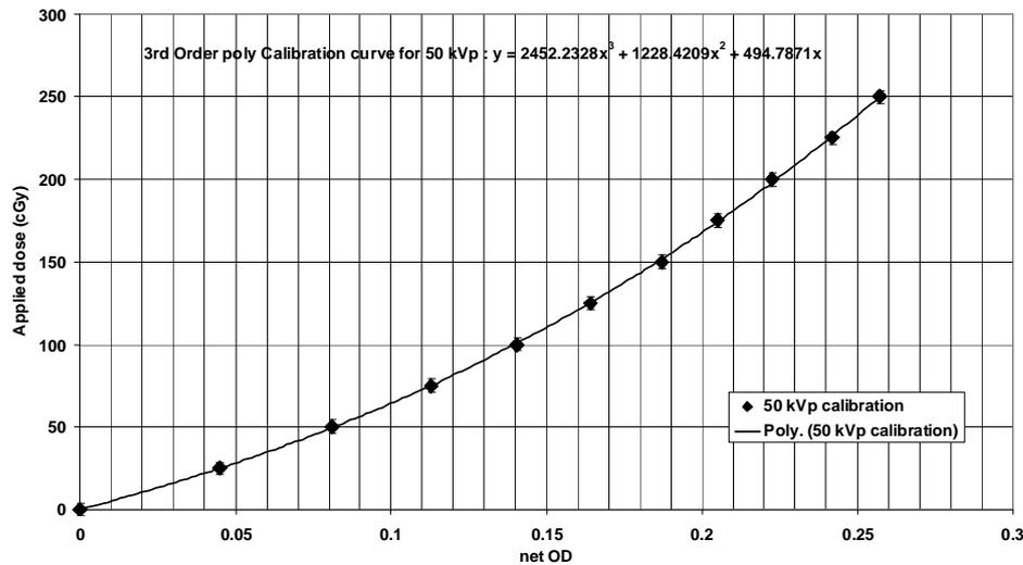
**Figure 1.** Example calibration curve for a 50 kVp x-ray beam irradiation using GAFCHROMIC™ EBT film. From results, a 3<sup>rd</sup> order polynomial function was found to accurately match experimental data for conversion of experimental OD to absorbed dose.
