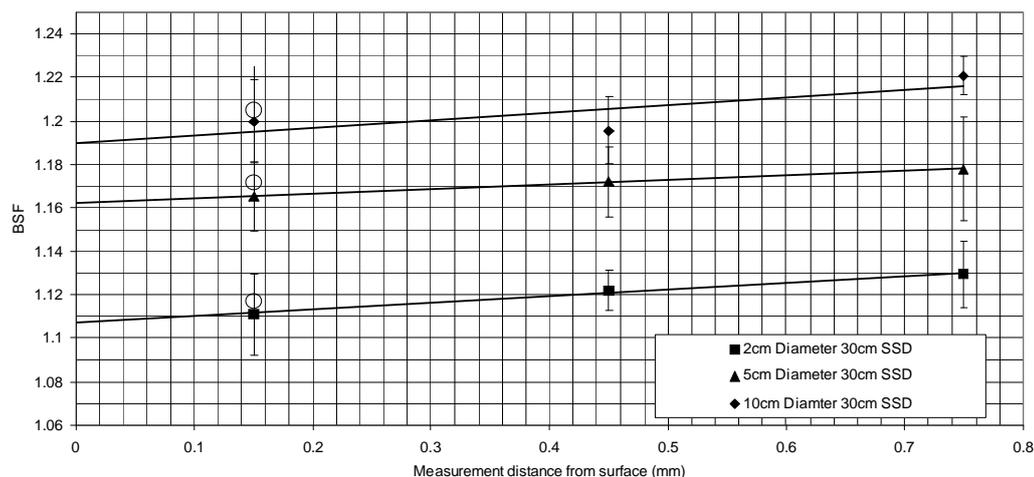
**Figure 2.** Example linear extrapolation of Backscatter factors for a 50 kVp beam field sizes 2 cm, 5 cm and 10 cm circle. The BSF values measured with a single film layer are shown as well (open circles). The solid lines represent the linear function fitted through the measured values that were used to extrapolate to zero thickness.
