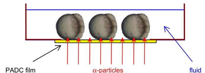
Fig. 2. The irradiation of the zebrafish embryos through the PADC-film based holder.
