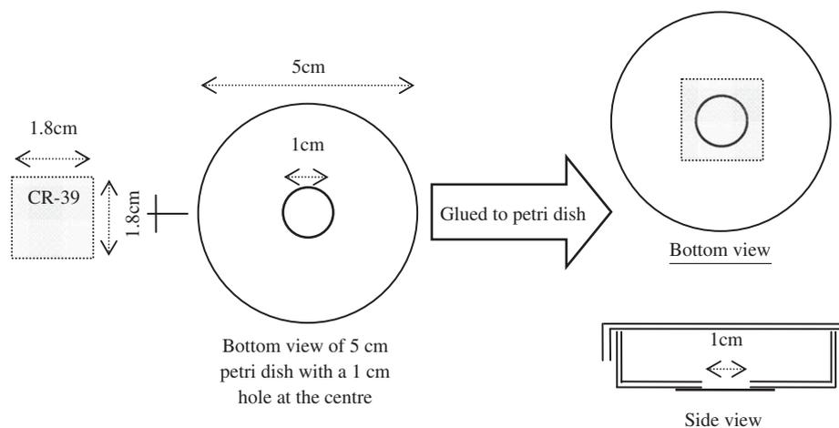
Fig. 1. Preparation of a custom-made PADC-film based holder by gluing a thin PADC film onto the bottom of a petri dish with 5 cm diameter and with a 1 cm hole drilled at the center of the bottom (Chan et al., 2006).
