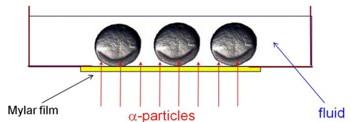
Fig. 1. Irradiation of 5 hpf zebrafish embryos with alpha particles through a Mylar film based holder.
